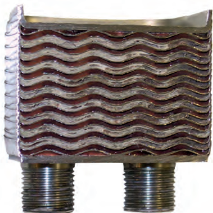
Heat exchanger is calcified
